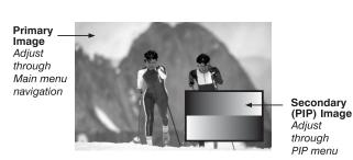
*NOTE: Disable PIP and Best Switching for Interlaced sources > 35kHz.*
